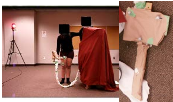
Figure 1 : Left : Setup with participant handling the ultrasound probe. Ultrasound machine was covered with cloth to avoid reflections and VICON camera. Right: Probe attachment with 3 markers.
