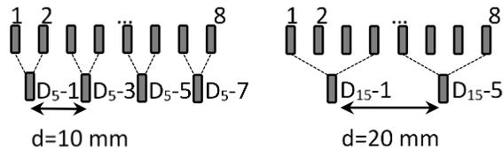
**Figure 2:** IED and ISD configurations: IED=5 mm and ISD=10 mm (left); IED=15 mm and ISD=20 mm (right).
