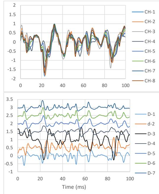
**Figure 3:** Monopolar (top) and bipolar (bottom) signals recorded from BRD (JA=60°; FL-1). Bipolar signals have 5 mm IED; D-1 = CH-1–CH-2, ... D-7 = CH-7–CH-8. Non-zero offsets have been added to the bipolar signals to separate the individual traces.
