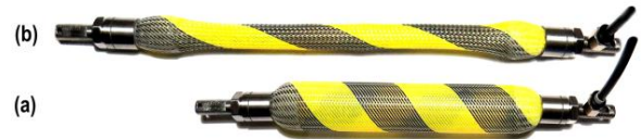
Fig.1. PAM prototype.(a) Pressurized state (b) Deflated state.
