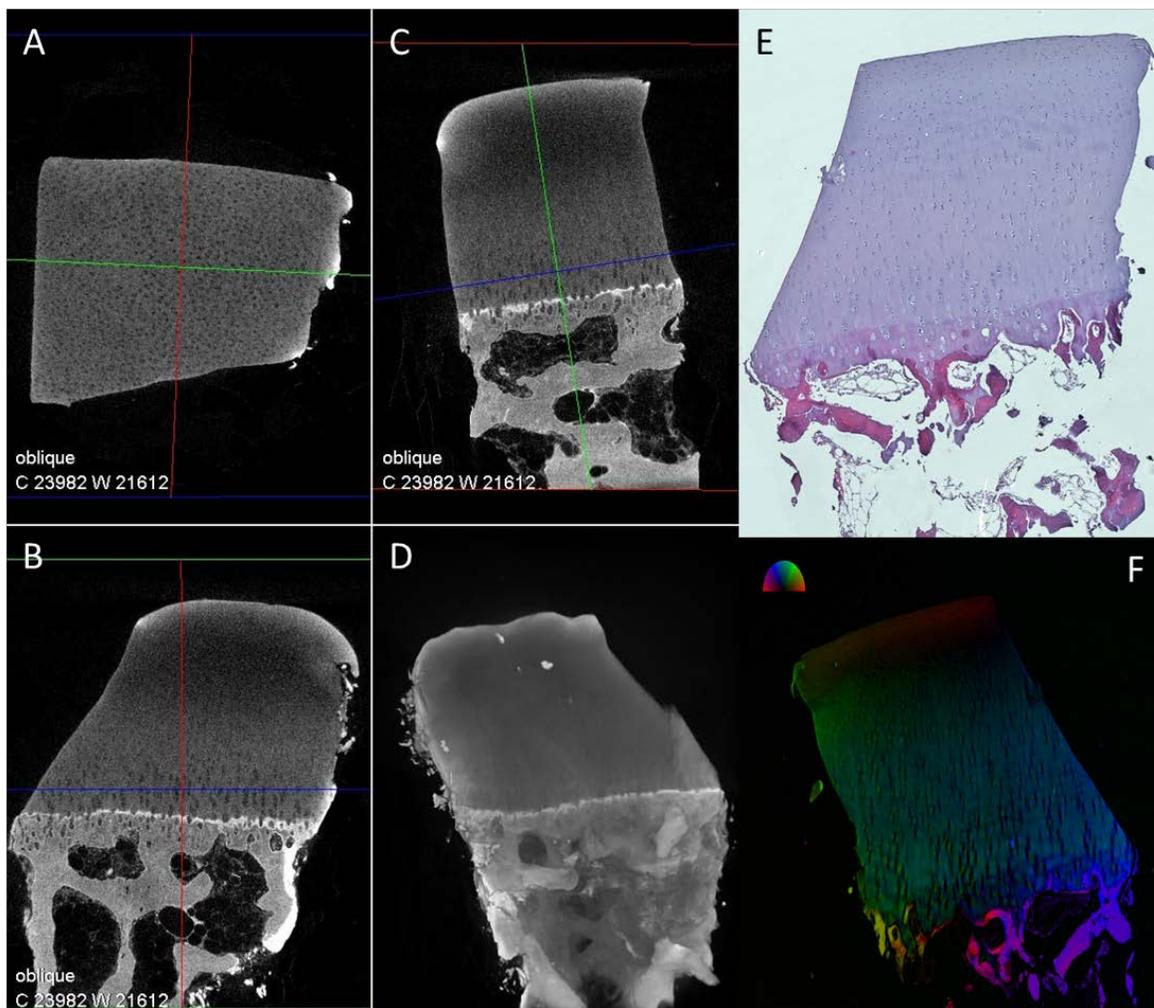
Figure 4: XRM images (3 orthogonal planes A-C and 3D view D) of the 91 hrs PTA-stained small ACB vs histology (E) & polarized LM (F).
