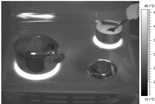
Figure 2: Thermal image of 4-burner stove top showing human activity (top-right) and thermal noise (top-left).
