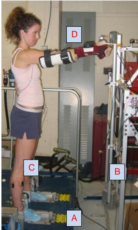
**Figure 1.** Side-on view of a typical subject executing a voluntary arm movement while standing on the actuator. **A.** Bilateral electro-hydraulic actuator fitted with two foot pedals and torque, position and load transducers. **B.** Aluminum target frame holding visual and audio cues, torque feedback meter and target switch. **C.** EMG surface electrodes on postural and focal muscles. **D.** Inclinometer used to measure arm angle.
