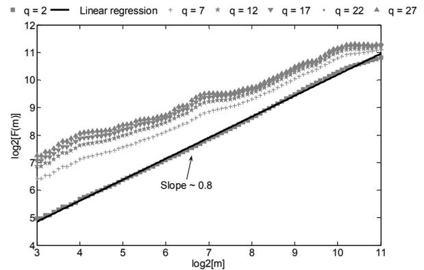
Figure 6: This segment of the signal has been collected 500 sec after the start of static contraction from subject 1 (MDN ~ 43 Hz). After random walk integration samples exhibit a high degree of mono-fractality which is also highly persistence (slope = 0.8) compared to non-fatigued case (slope = 0.5).
