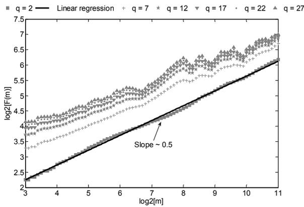
Figure 2: Analysis of simulated fractional Brownian motion after random walk integration. The slope accurately characterizes the time series.
