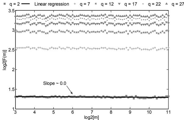
Figure 1: Analysis of simulated fractional Brownian motion before random walk integration. The slope is not informative.
