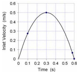
Figure 3: Variation in time of the inlet velocity profile.
