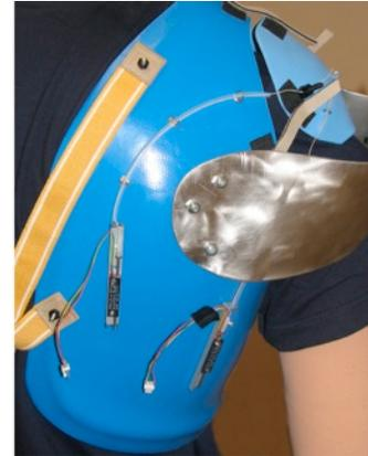
Figure 5: Experimental Bypass Socket with Linear Transducer Inputs used for the Evaluation of the Vector Projection Algorithm
