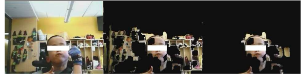
Figure 5: An image processing example. Left: Original frame. Middle: Frame after skin colour segmentation. Right: Segmentation with background subtraction.
