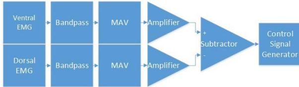
Figure 2: 2-channel EMG signal processing diagram
