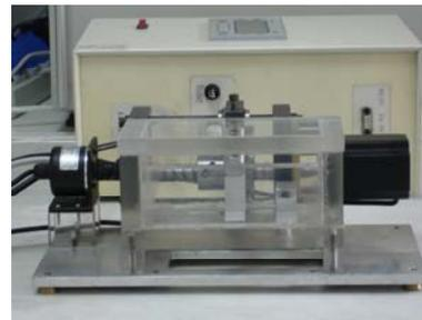
Figure 1: cyclic strain exertion apparatus
