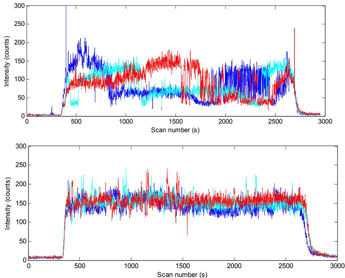
Figure 6: Top 3 traces show direct infusion of Glufib analyte on an unenclosed instrument. Bottom 3 traces show the same experiment on the same instrument with the new enclosure.
