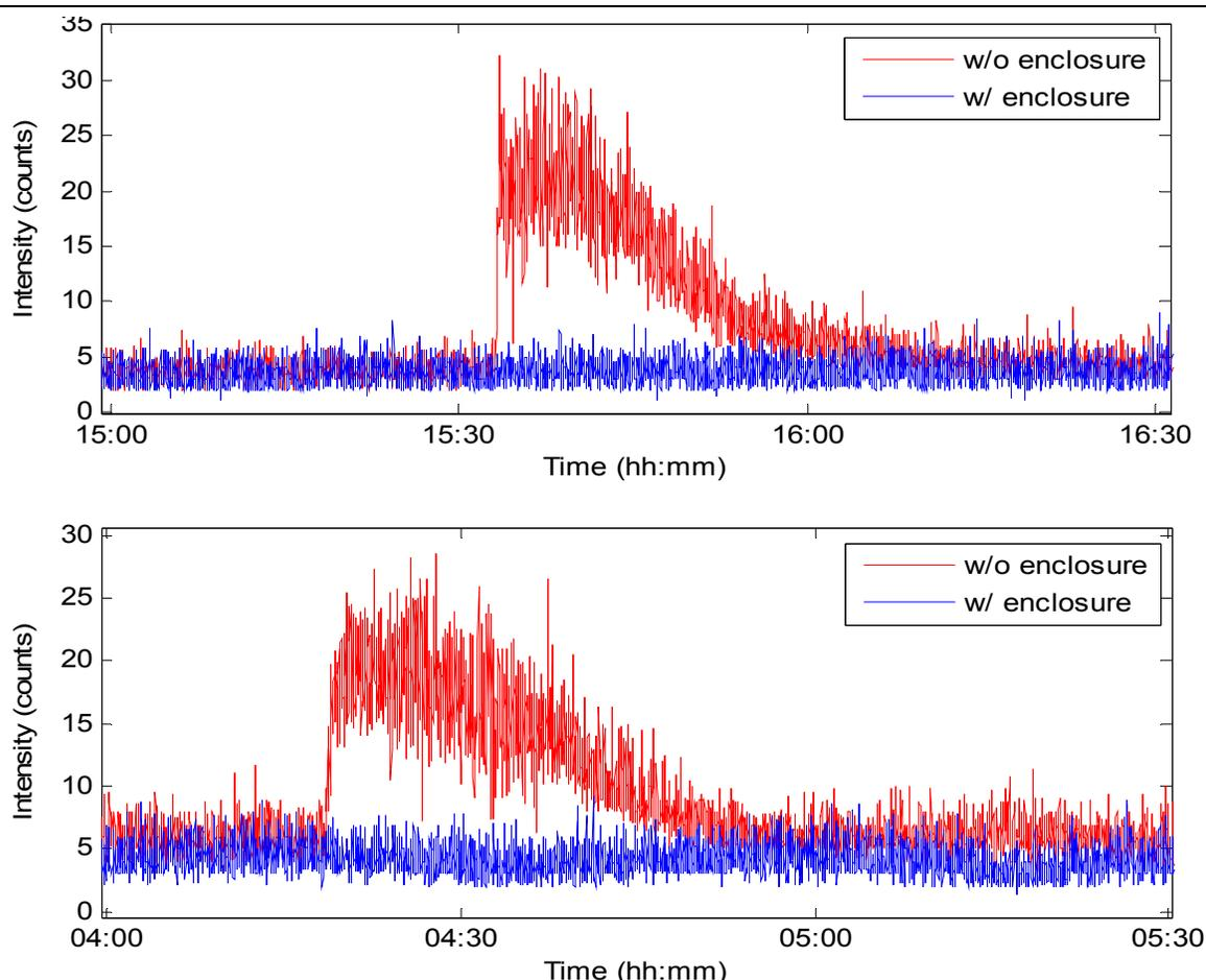
Figure 5: Two examples of a 30 minute burst of contaminant on an unenclosed instrument [Red trace], and no corresponding increase in the enclosed instrument [Blue Trace].
