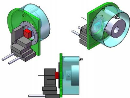
Figure 3: CAD rendering of designed enclosure, with spray stage and mass spectrometer inlet
