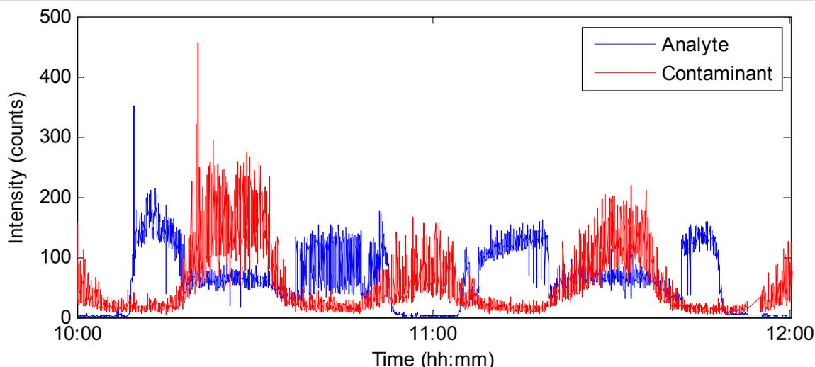
Figure 1: Infusion of analyte at  $\sim 785$   $m/z$  [BLUE] being cannibalized by contaminant signal at 355  $m/z$  [RED].
