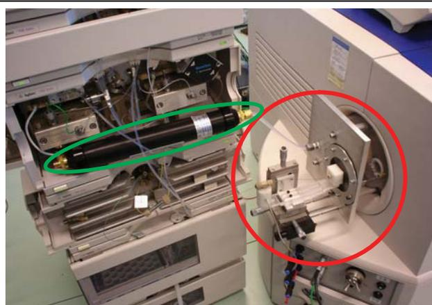
Figure 4: Enclosure assembly (red) mounted on mass spectrometer, activated carbon filter (green)
