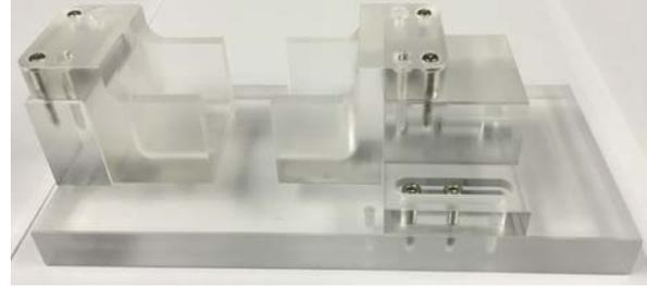
Figure 3: Specimen preparation jig
