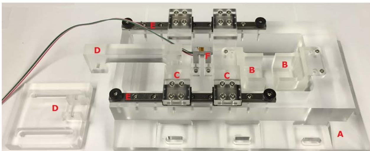
Figure 1: Device: A = base; B = bone pots; C = carriages; D = attachments for linear drive; E = linear rail guides; F = load cell.
