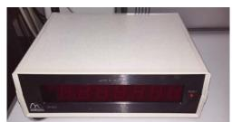
Figure 5: Siskiyou DR1000 Digital Readout
