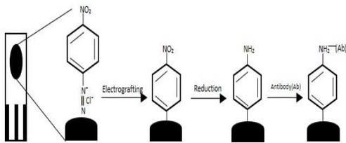
Fig1: Functionalization of the electrode with immobilized antibody
