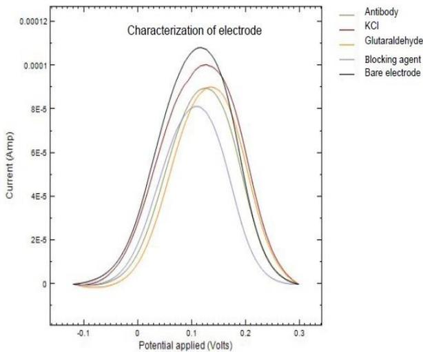
Fig 2. Characterization of the electrode after each stage of surface modification.
