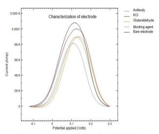
Fig 2. Characterization of the electrode after each stage of surface modification.
