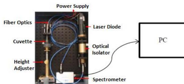
Figure 1: Components of the sensor system
