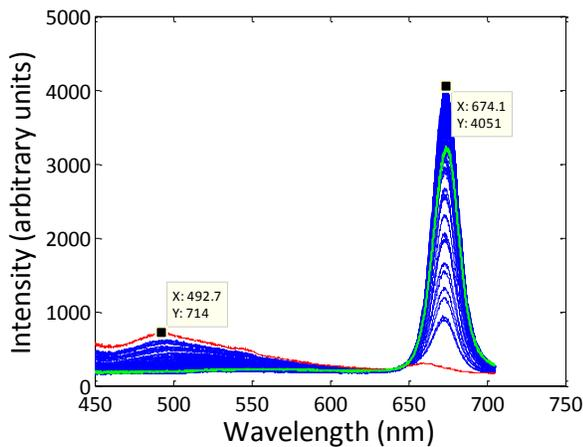
Figure 2: Fluorescence spectra of 100 samples: green for EVOO, blue for adulterated oil, red for sunflower oil
