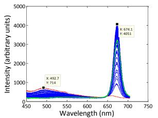
Figure 2: Fluorescence spectra of 100 samples: green for EVOO, blue for adulterated oil, red for sunflower oil
