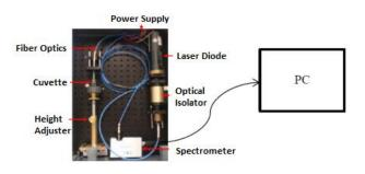
Figure 1: Components of the sensor system
