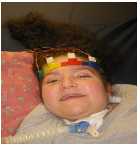
Figure 1: The participant wearing the headband with four accelerometers on the forehead for initial detection of eyebrow movements.
