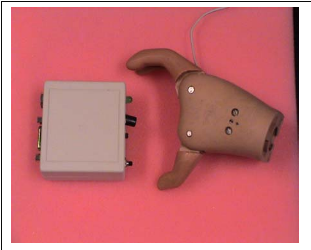
Figure 2: Wireless base station prototype for connection with computer and graphical user interface software.
