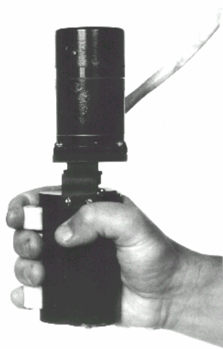
Figure 1. -- Device for increase and rehabilitation of strength of hand and fingers
