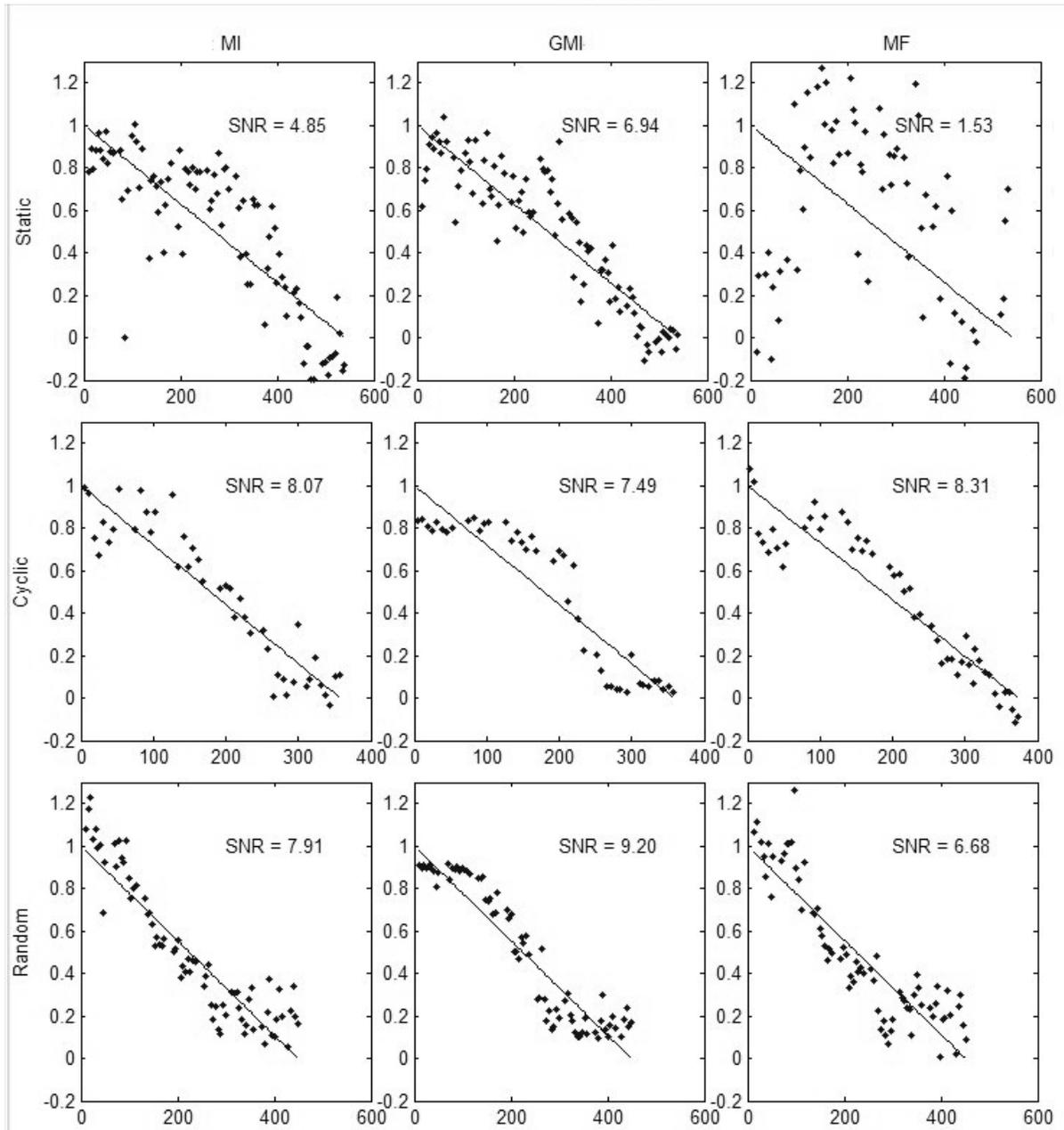
Figure 1: GMI, MI and normalized MF fatigue estimates from test data of participant 7 under static, cyclic and random contraction conditions
