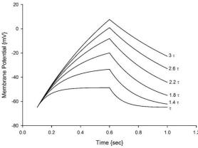
Figure 4: Comparison of time constant and membrane potential among six different ion channel density.
