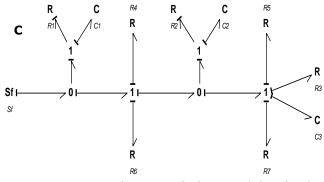
Figure 1: General view of the model. A) The axons and dendrites of a neuron and thin tube of membrane; B) An electrical circuit representing a one-dimensional nerve:  $R_i$  and  $R_e$  are the intracellular and extracellular resistances per unit length ( $\Omega/m$ ),  $R_m$  is the membrane resistance and  $C_m$  is the membrane capacitance per unit length (F/m) [17]; C) The bond graph model of the neuron.
