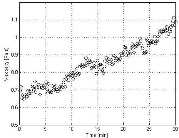
Figure 1: Viscosity of sample 5 is plotted as a function of time at a constant shear rate of 0.05 s<sup>-1</sup>.
