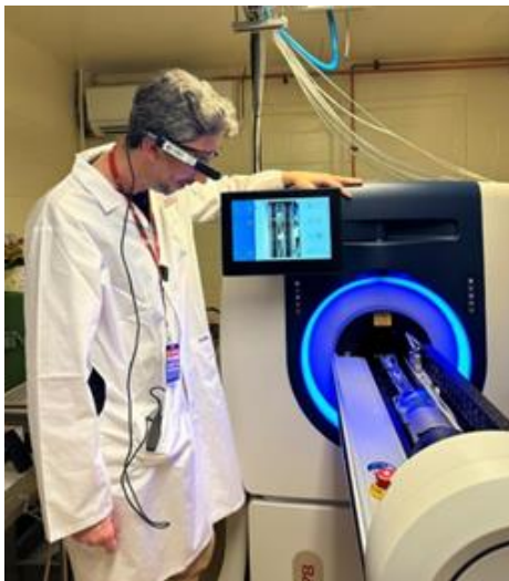
Fig. 1 Troubleshooting PET/CT scan equipment using TeleVU glasses
