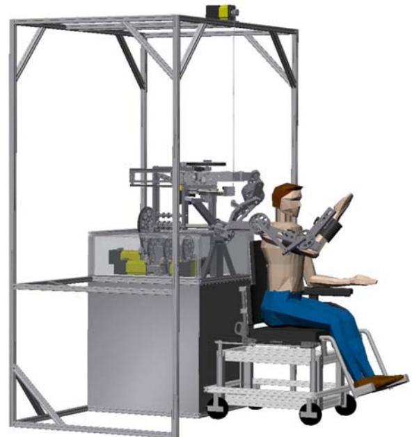
Figure 1: A CAD drawing of a user with MEDARM. In addition to the MEDARM robot itself, the system consists of a support structure, an adjustable chair, and an external gravity compensation system.
