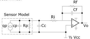
Figure 2: Circuit model of the piezo-sensor and the signal conditioning circuit.
