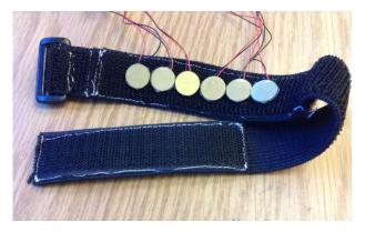
Figure 1: Photograph of the piezo sensor array wrist apparatus. Shown are the 6 piezo disc sensors, the soft Velcro strap, and the hook side Velcro for tightening.
